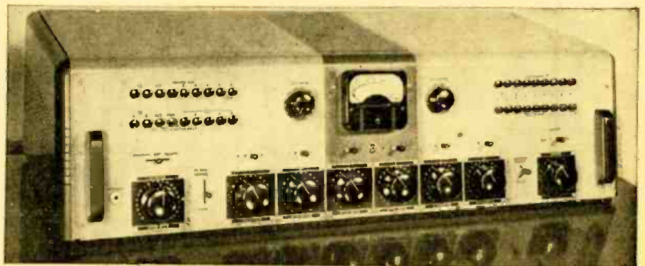
Appearance of the RCA 76-B2 Studio Control Console, a typical and commonly-used type.
